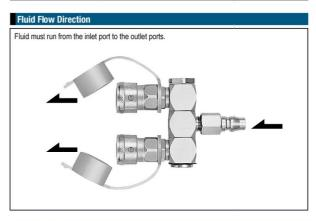
Interchangeable with plugs of HI CUPLA models 10, 17, 20, 30 and 40. Interchangeable with each models of NUT CUPLA series and HI CUPLA series. Please see page 19 for "HI CUPLA Series Interchangeability".
